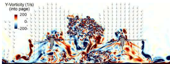
Fig. A5. Slice cutting through side-by-side H/D = 0.5 3.0R separation IGE rotor hubs colored by Y-vorticity (simulated with C/8 sized interrotor grid elements).
