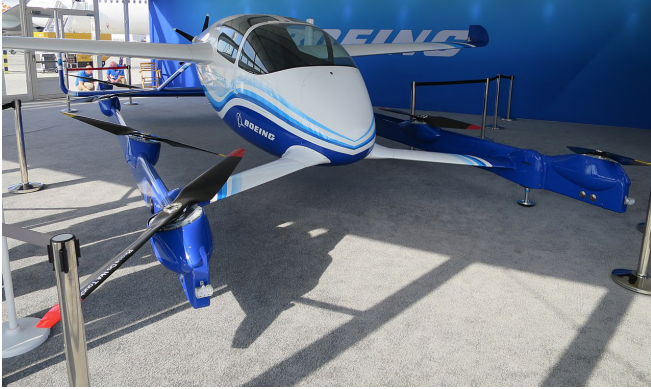
Figure 1. Laterally canted rotors on the Boeing PAV (Ref. 9)
