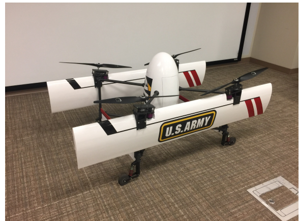
Figure 1. CRC-20 Quad-Rotor Biplane Tailsitter (Ref. 9) autonomously necessitate a mechanism to avoid obstacles and perform maneuvers within cluttered environments. Thus, incorporating obstacle avoidance into path planning methodologies and control architectures for transitioning UAS is crucial to their eventual real-world application.
