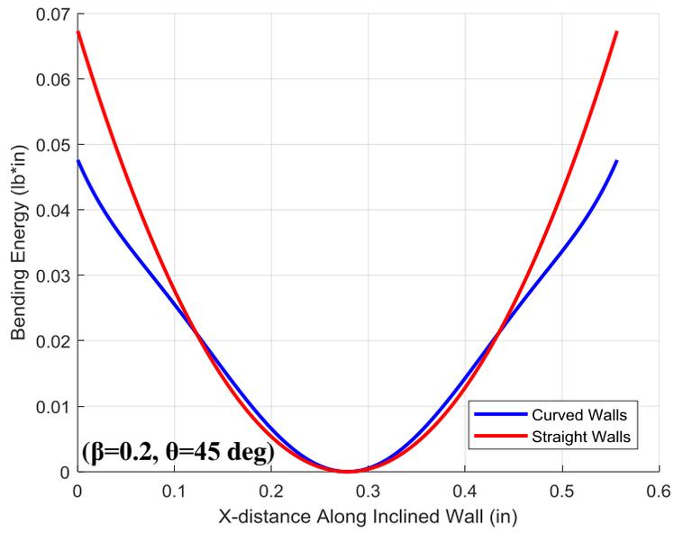
**Figure 20 – Bending energy distribution for straight- and curved-wall cells under 10 lbs load in the y-direction**
