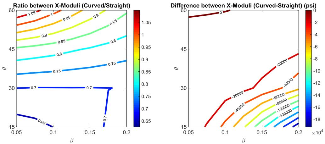
Figure 9 – Ratio and differences between x-modulus between curved- and straight- walled cells
