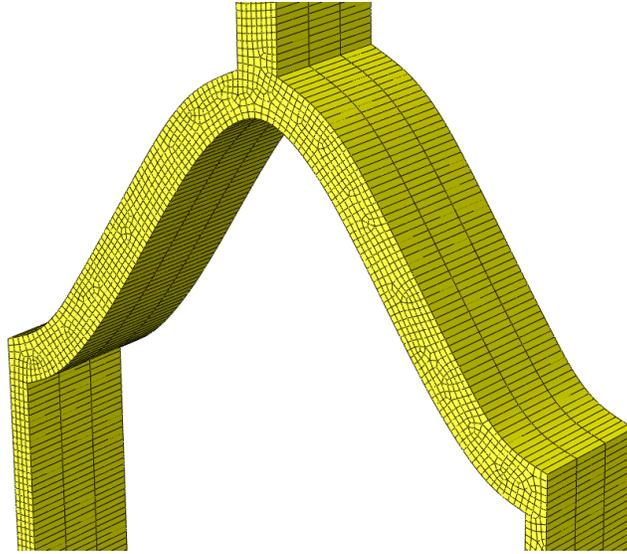
Figure 3 – Sample of 3D finite element mesh ( $\beta=0.1$ ,  $\theta=45$  deg)
