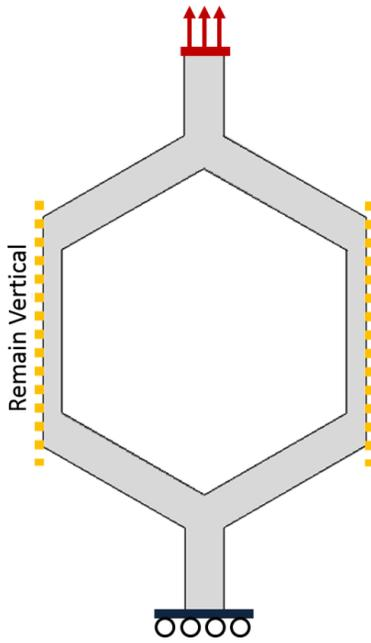
Figure 4 – Sample boundary conditions enforced on generic unit cell undergoing vertical extension
