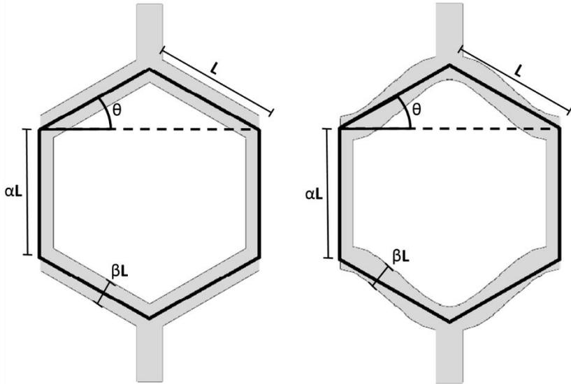
**Figure 2 – Nondimensional parameters applied to straight- and curved-wall cellular lattices**
