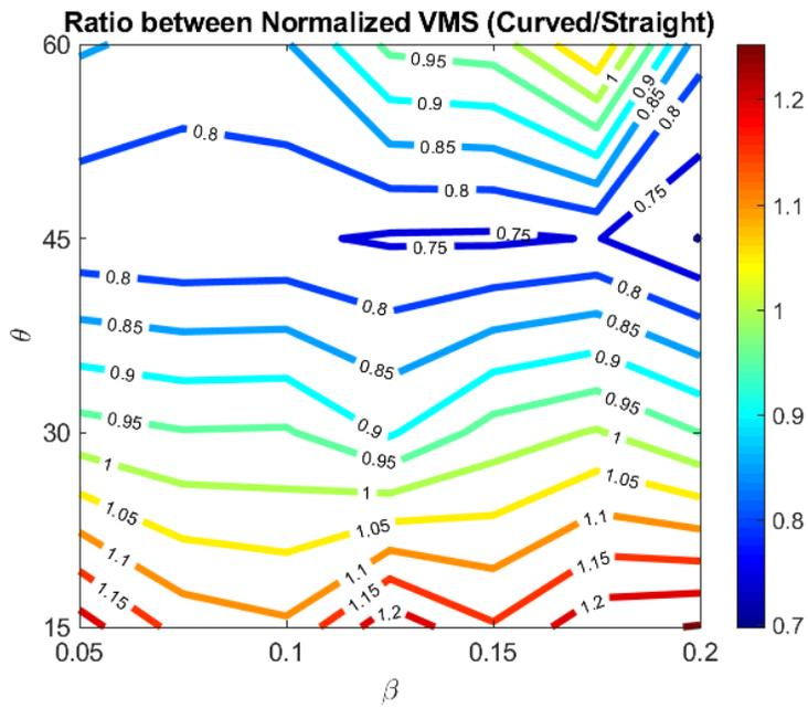
Figure 13 – Ratio between normalized Von Mises stress for curved- and straight-wall cells in y-direction loading
