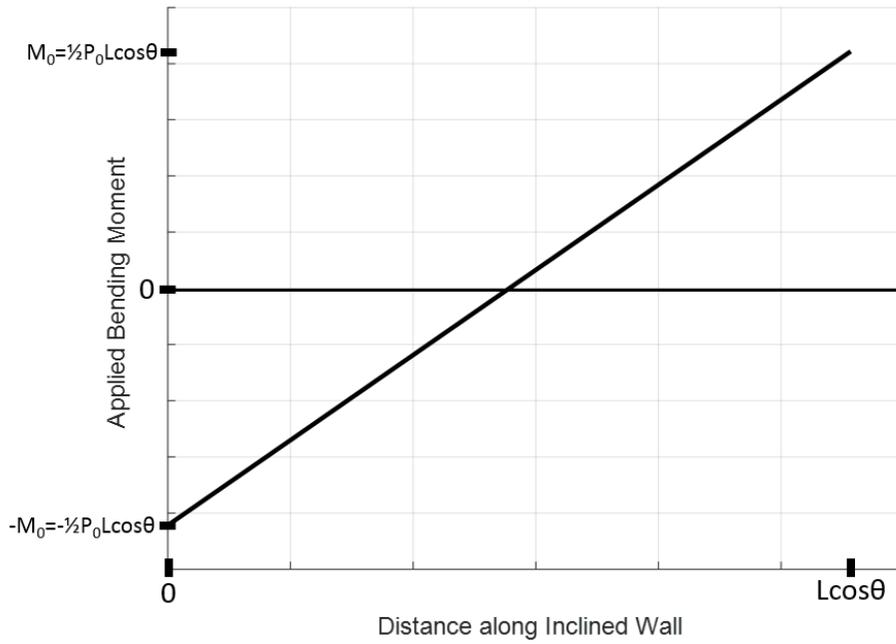
**Figure 21 – Bending moment along inclined wall length**
