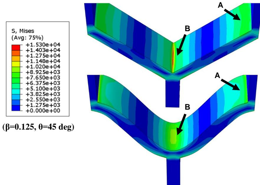
Figure 11b – Von Mises stress for straight- and curved-wall cells in y-direction loading
