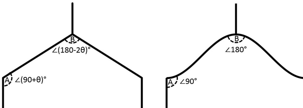
Figure 10 – Comparison of junction angles for straight- and curved-wall lattices
