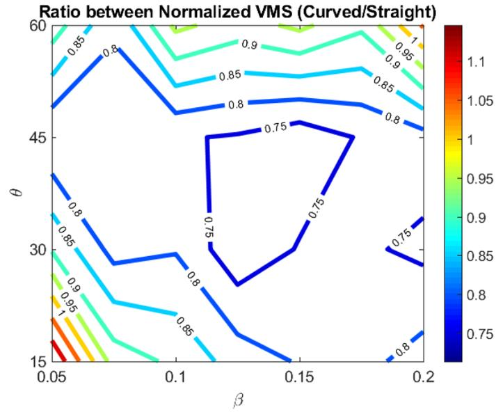
Figure 12 – Ratio between normalized Von Mises stress for curved- and straight-wall cells in x-direction loading
