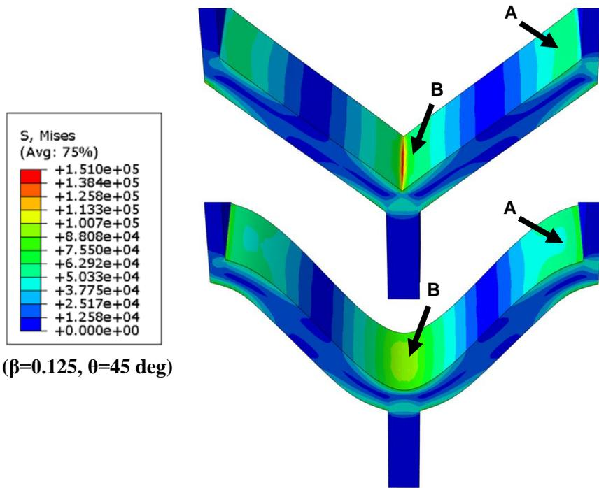
Figure 11a – Von Mises stress for straight- and curved-wall cells in x-direction loading
