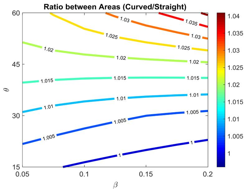
Figure 7 – Ratio between frontal area of cells with curved and straight inclined walls
