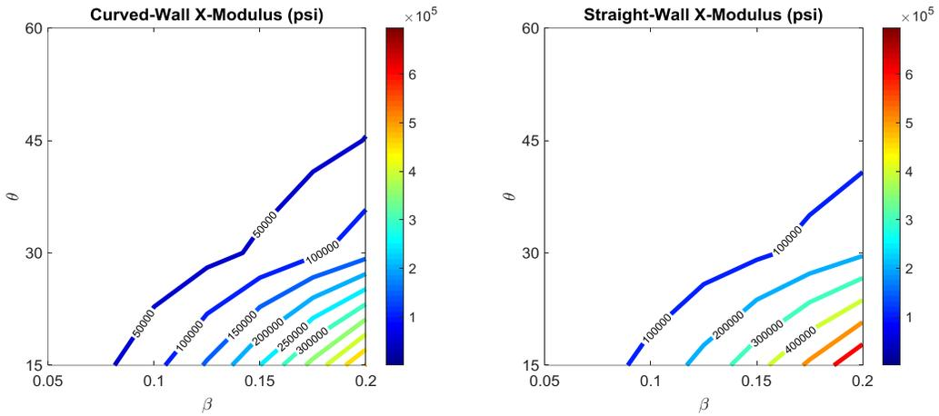
Figure 8 – System modulus for various cell geometries under x-direction loading
