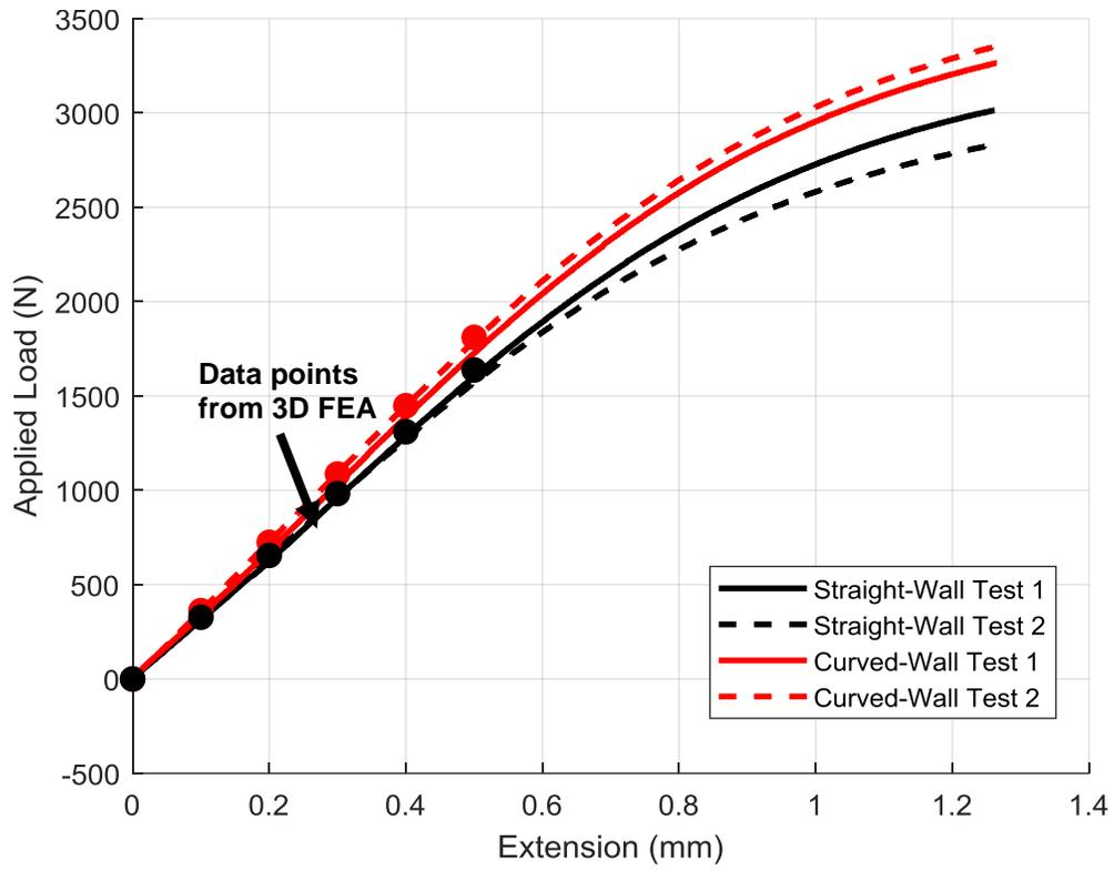
**Figure 16 – Load versus displacement curve for tensile samples**
