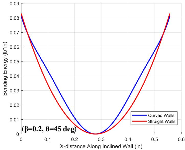
Figure 19 – Bending energy distribution for straight- and curved-wall cells under 1% strain in the y-direction
