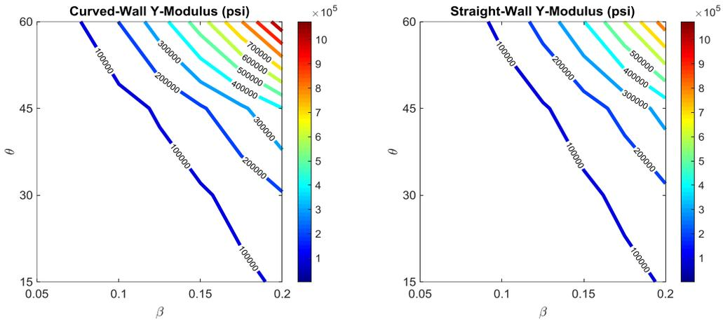
Figure 5 – System modulus (psi) for various cell geometries under y-direction loading
