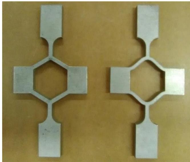
Figure 15 – Straight- and curved-wall cells waterjet cut from Aluminum
