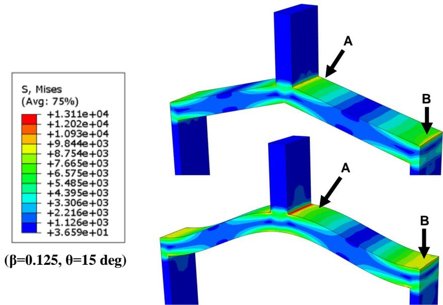
Figure 14 – Von Mises stress for straight- and curved-wall cells in y-direction loading
