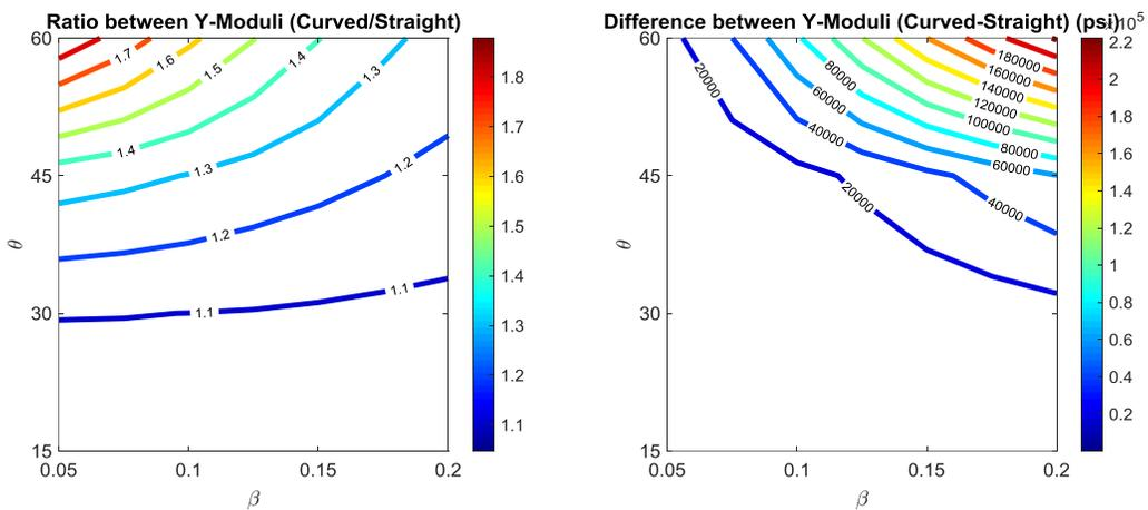
Figure 6 – Ratio and differences in y-modulus between curved- and straight- walled cells
