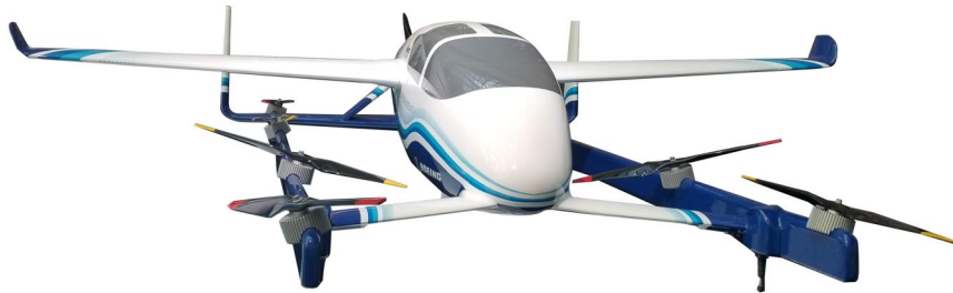
Fig. 1 Laterally canted rotors on the Boeing PAV. Reprinted with permission from the Vertical Flight Society [17].
