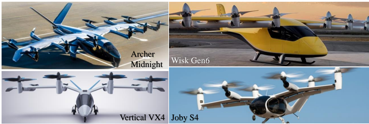
Fig. 2: eVTOL configurations using tilting prop-rotors
