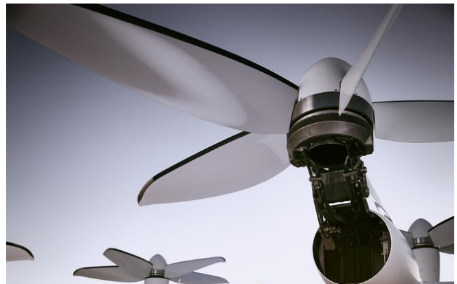
Fig. 1: High-solidity rotors on the Joby S4
