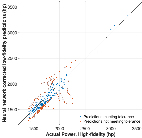
Figure 9: Actual vs predicted power of testing dataset, evaluated using initial ANN-based correction model at 150 kts
