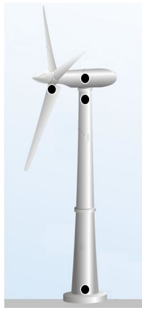
Figure 7. Monitored locations: blade root, nacelle, tower top and tower base (shown in dots).
