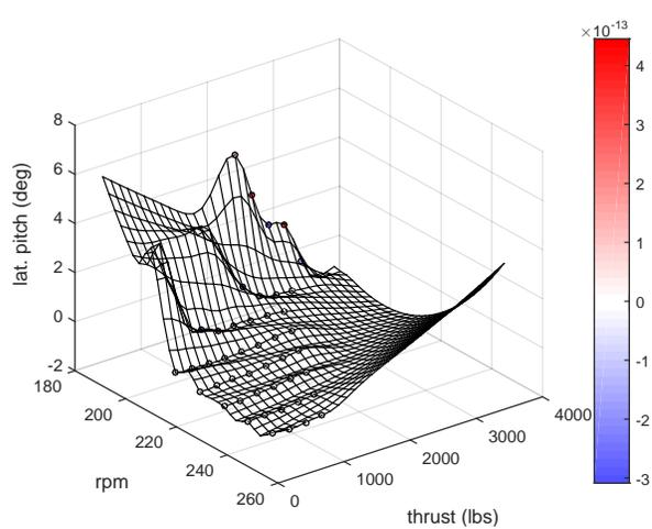
**Fig. 15. Lateral pitch data vs. response surface model, Kriging (fixed stab)**
