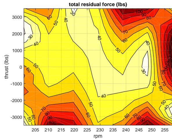
**Fig. 8. Residual force magnitude from response surface approximated trim**
