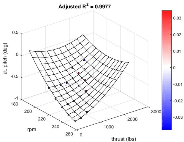
**Fig. 13. Lateral pitch data vs. response surface model, truncated set of trim states (fixed stab)**
