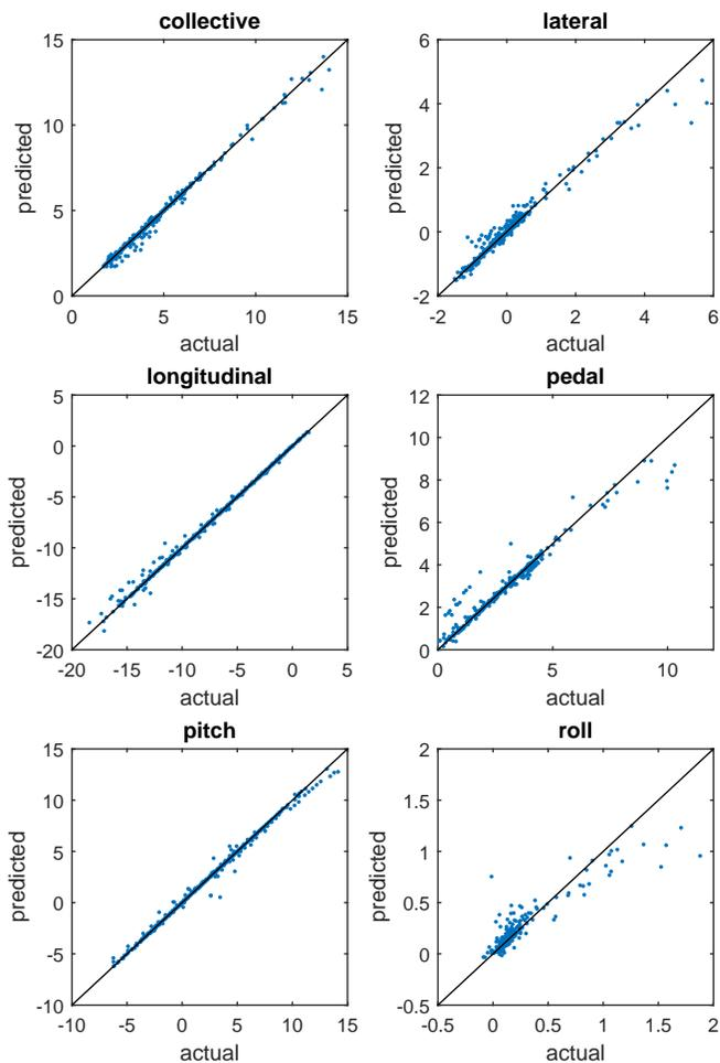
**Fig. 14. Comparison of actual to predicted control values using a Kriging model**
