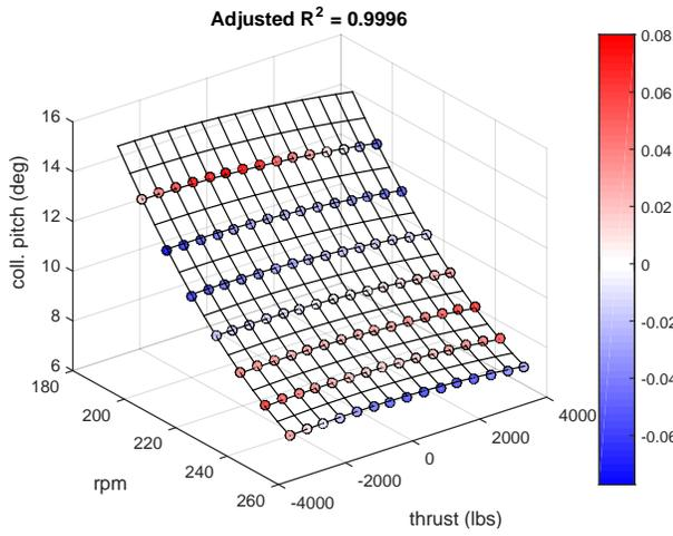
Fig. 1. Collective pitch data vs. response surface model
