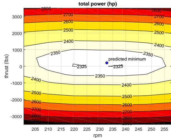
**Fig. 19. RCAS simulation of power with predicted minimum power labeled**
