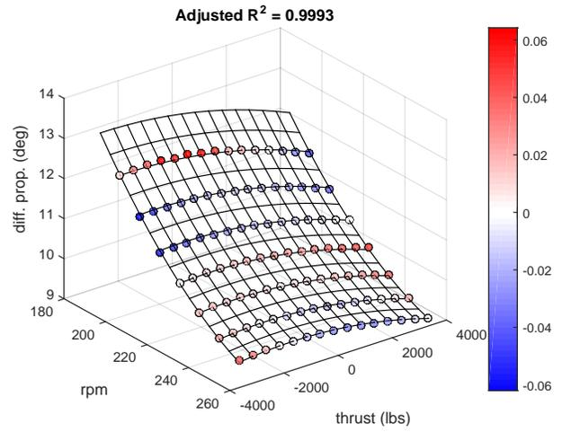
Fig. 4. Diff. prop. pitch data vs. response surface model
