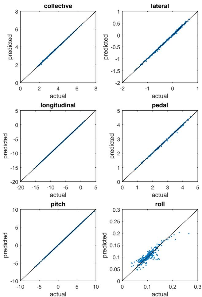
**Fig. 12. Comparison of actual to predicted control values after eliminating outlier data**
