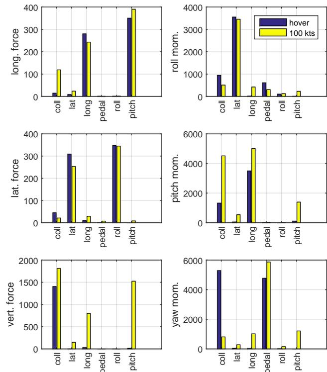
**Fig. 18. Control sensitivities in each force and moment direction over three flight speeds (lbs/deg or lbs-ft/deg)**
