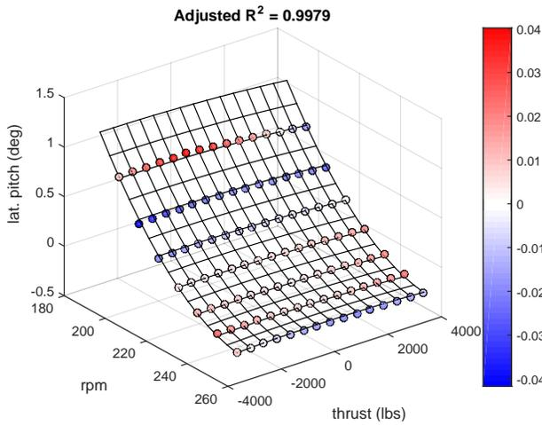
Fig. 2. Lateral pitch data vs. response surface model
