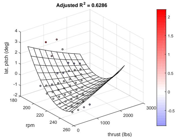
Fig. 11. Lateral pitch data vs. response surface model, all trim states (fixed stab)
