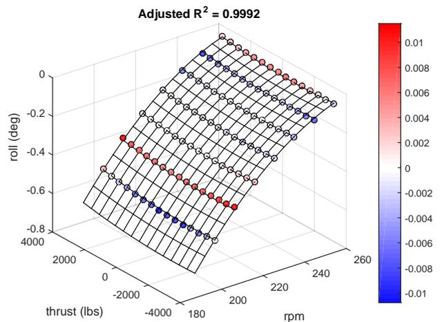
Fig. 6. Roll attitude data vs. response surface model
