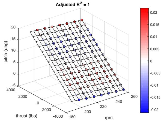
Fig. 5. Pitch attitude data vs. response surface model
