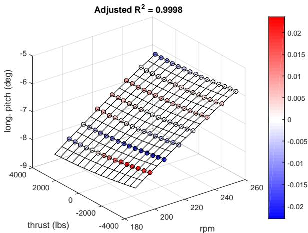
Fig. 3. Longitudinal pitch data vs. response surface model
