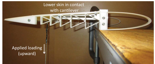
Fig. 20 Prototype inverted to measure tip displacement under “upward” load.
