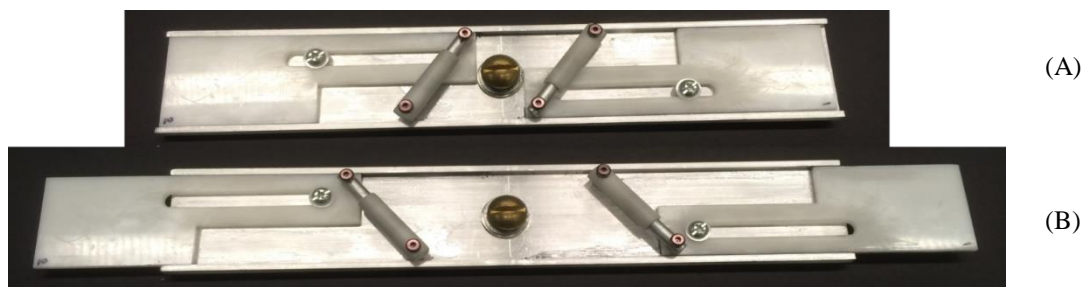
Fig. 6: Prototype rotor with inserts in the (A) retracted and (B) extended configuration.
